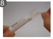
Un-cap liquid tube. Put white swab into the same tube and break swab shaft off at the pre-moulded breakpoint.
